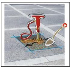
A trench under the asphalt should be made according to the best practices between the excavation for the lost casing and the inspection hole (or control system). This trench should contain a (JANOLENE type) protective geotextile sheath Ø 100 mm.
